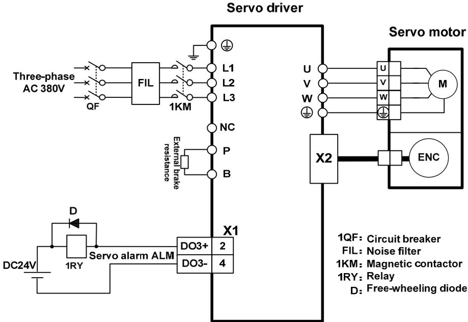
Note: TH50、TH75 have no internal brake resistance and need to be connected with external brake resistance.
