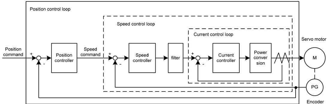
Theoretically, the bandwidth of the inner control loop must be higher than that of the outer control loop. Otherwise the whole control system will be unstable and cause vibration or poor response.
