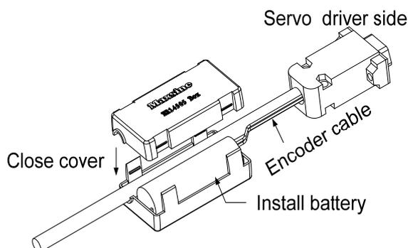
**Note: Please set the battery unit on the servo driver side. Please set the battery unit on either side of the servo driver.**
