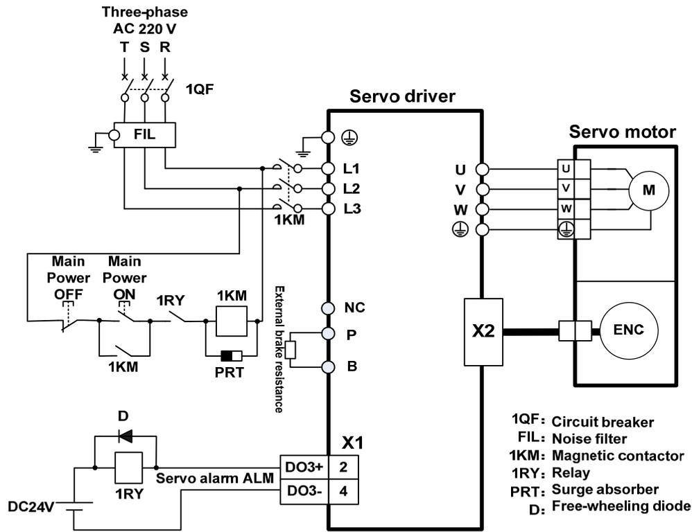
Note: TL55 has no internal brake resistance, so it needs to be connected to external brake resistance.
