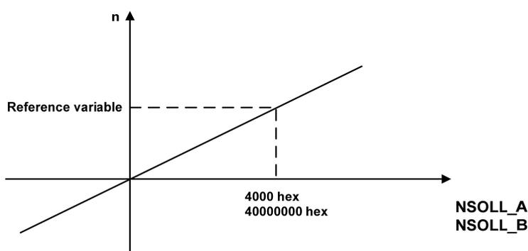
As shown in the figure above: Linearly normalized values, 0% corresponds to 0, for N2 type data, 16 bits are used, and 100% corresponds to 214(i.e. 0x4000); For N4 type data, make the 32-bit representation, 100% corresponding to 230(that is, 0x40000000).
