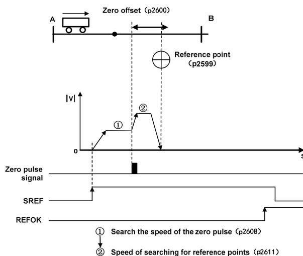
Back to the reference point in the process of related parameters as shown below:
