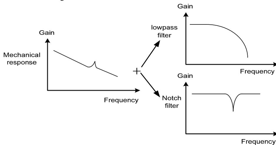
The characteristics of the two filters are:
