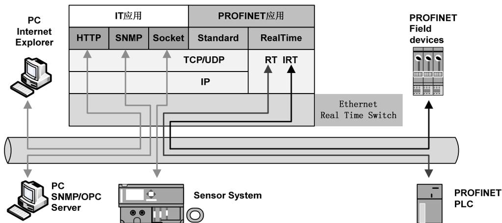
PROFINET provides two kinds of real-time communication, PROFINET IO RT and PROFINET IO IRT.
