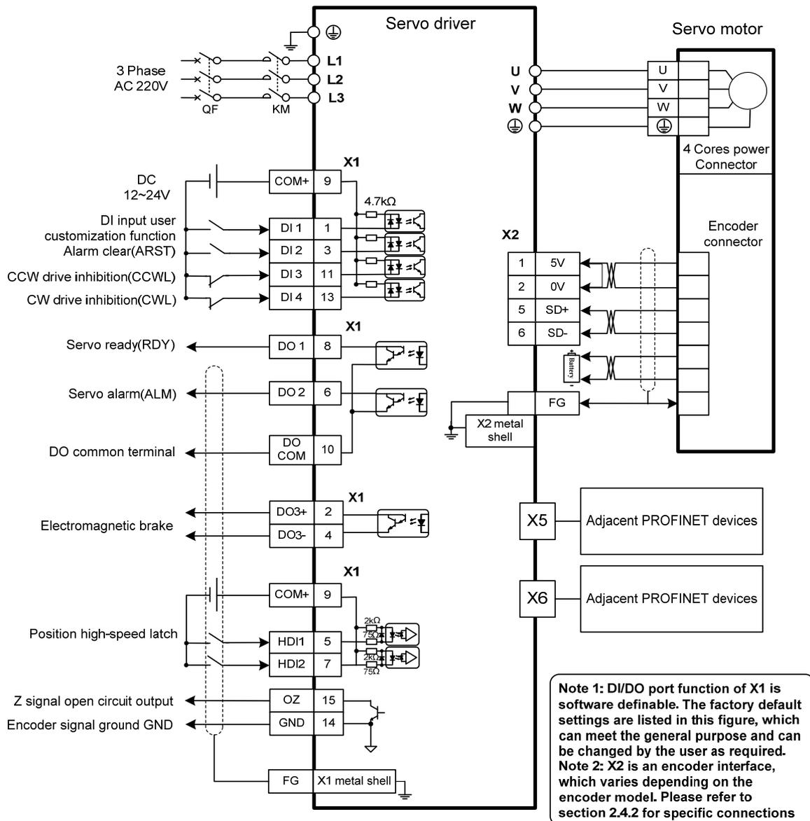
Note: The above wiring diagram takes TL15 as an example.
