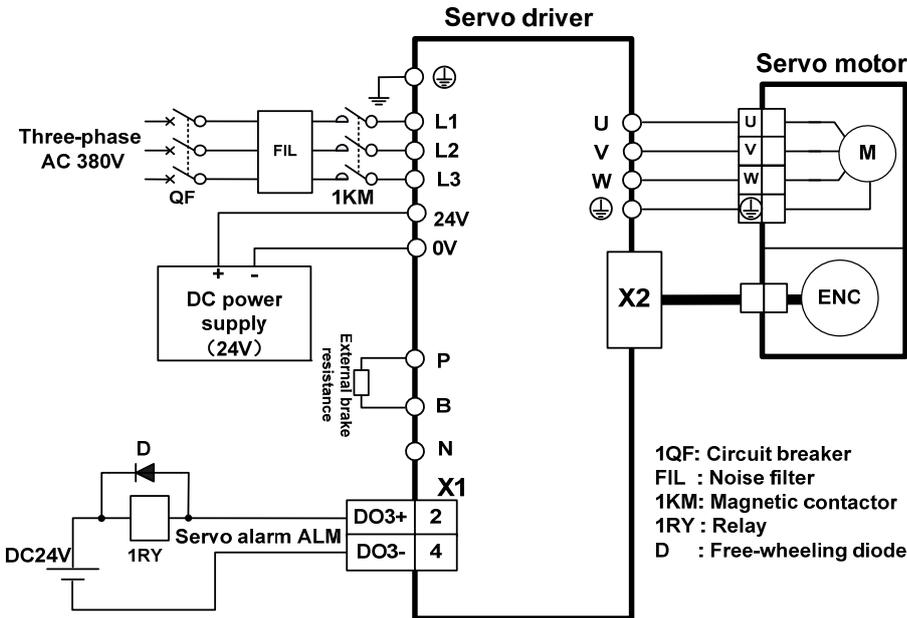
Note: TH90、TH110、TH150 have no internal brake resistance, and need to be connected with external brake resistance for use.
