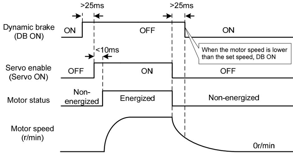
Note: Model TL04/TL08/TL10 comes with an onboard dynamic braking relay, which only supports internal dynamic braking function and is controlled by P083, without external dynamic braking function; Other models do not have onboard dynamic brake relays, only external dynamic brake functions.
