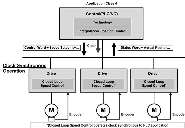
Application class generally do not need the speed setting of the AC4 channel slope function generator, the following chart from out of the station equipment the speed setting of the simplified channel module function, to the speed set point STW1.5 channel has no effect.
