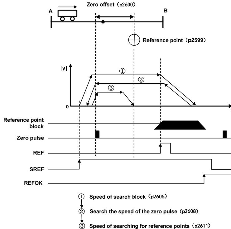
Back to the reference point in the process of related parameters as shown below
