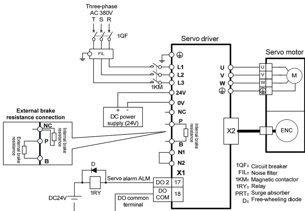
Note 1: GH130 is a built-in braking resistor, which can meet the general situation.
