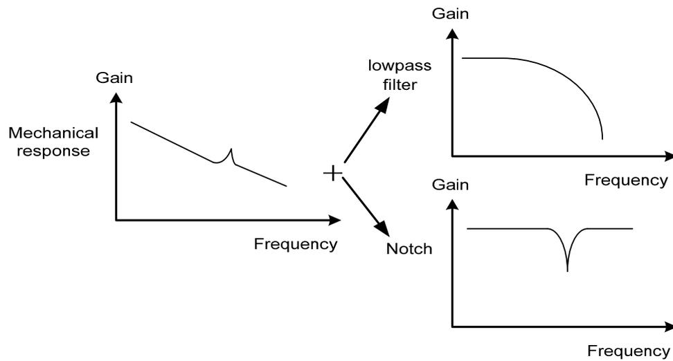
The characteristics of the two filters are:
