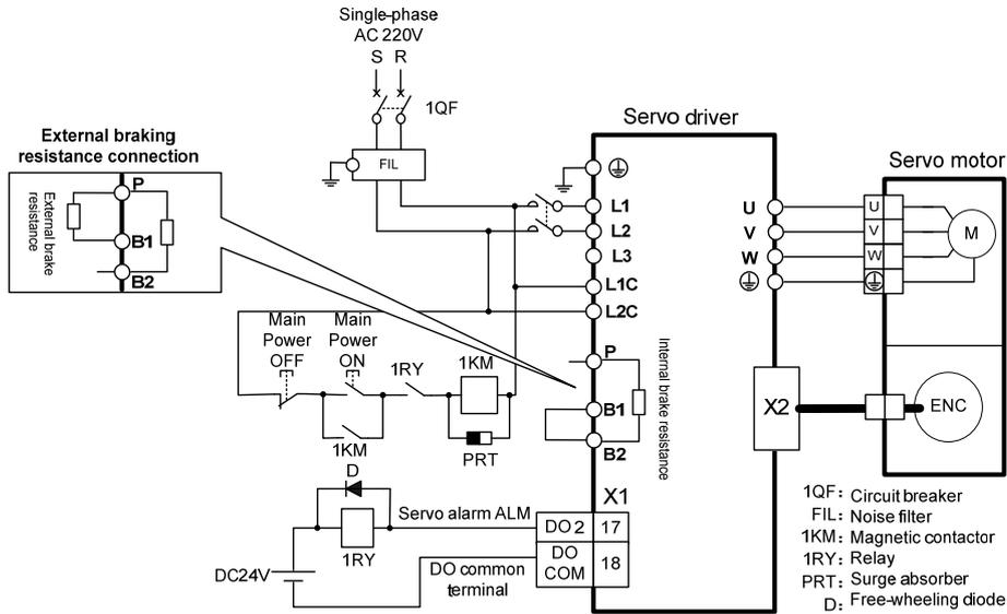
Note: GL1A0 has no internal braking resistor, so it is generally unnecessary to connect the braking resistor.
