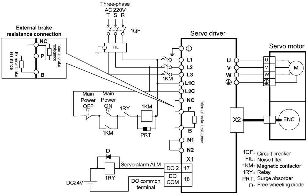
Note: GL240 has no internal brake resistance and needs to be connected to external brake resistance.
