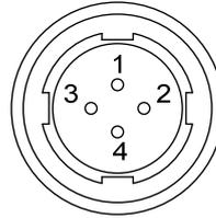
40/60/80 motor power plug    110/130/180 motor power plug
