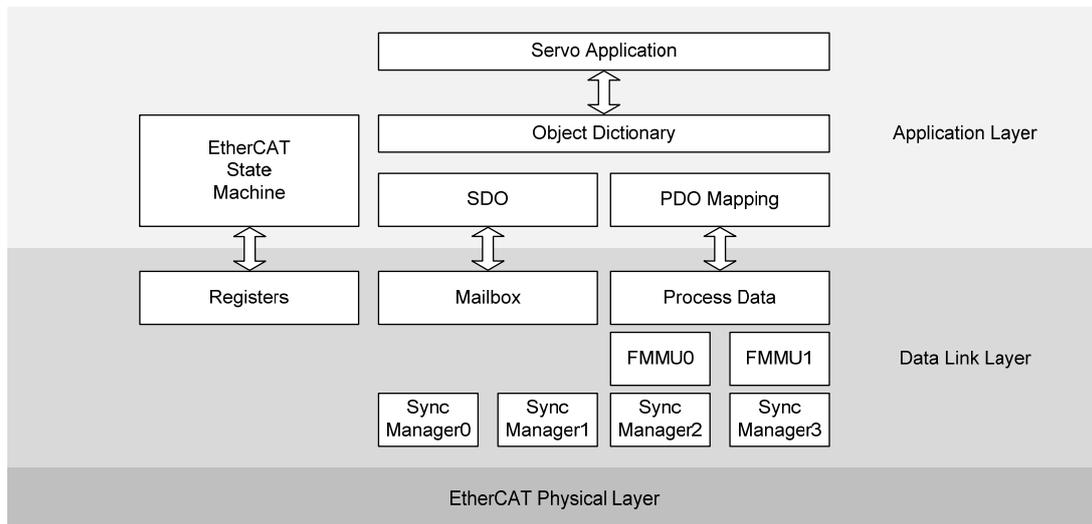
The drive adopts the shape of the CiA 402 drive. The Object Dictionary of the application layer includes the application data and process data interface, as well as the PDO mapping information between application data.
