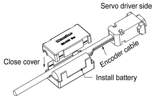
**Note: Do not set the battery unit on both sides of the servo drive. Please set the battery unit on either side of the servo driver.**
