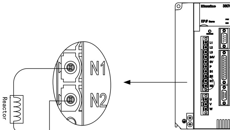
Note: Only GL190, GL240, GH2A0, GH3A5, GH5A4, GH8A5, GH130, GH170 and GH210 servo drivers have the function of connecting external reactors.
