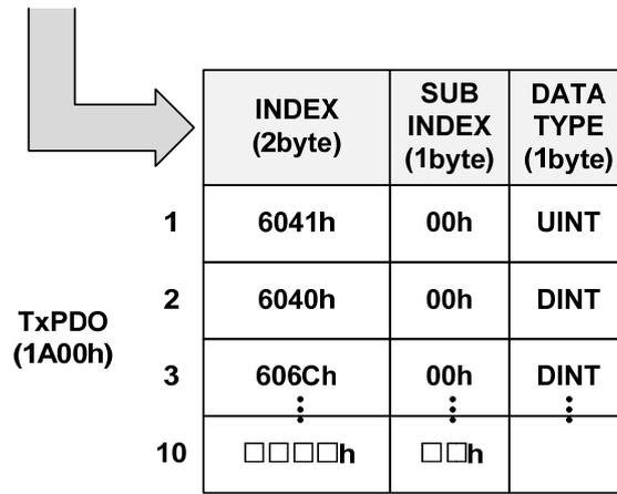
SyncManager can consist of several PDOs. SyncManagerPDO Assign Object (RxPDO: 1C12h, TxPDO: 1C13h) displays the relationship between SyncManger and PDO.
