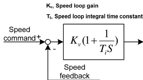
P018 can choose the speed controller structure. 0 is the IP regulator, 100 is the PI regulator, 1~99 is the PDFF regulator. If the parameter value of P018 is too large, the system has high frequency response; if the parameter value is too small, the system has high stiffness (resistance to deviation); if the parameter value is too small, both frequency response and stiffness are considered.
